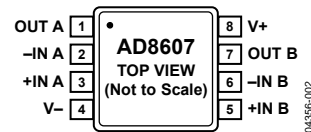
Figure 2. 8-Lead MSOP (RM Suffix)
